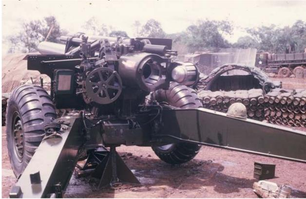
One of six 155mm howitzers in F Btry. Notice the gun balanced on the pedestal. One man could easily move the gun in this setup. Once pointed in the right general direction the XO would lay the gun in the exact direction, the gun would be jacked up and made ready to fire. Speed and accuracy was our goal. This howitzer shot the 50,000<sup>th</sup> round.
